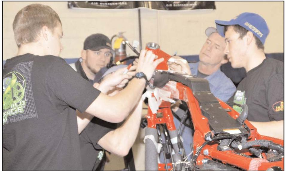
*In the top photo, Casey Evans, left, and Corey Aga, right, install the wiring harness onto the frame under the direction of Nick and Randy Cramer of Dakota V-Twin.*
